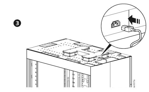
**Note:** Using one of the supplied power cords, connect the female end to one of the input sockets on the rear of the unit. Plug the male end into a UPS or other socket that provides protected power.
