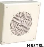
**Description** Bogen's MB8TSQ and MB8TSL speakers feature an all-steel surface-mounted enclosure with an 8" cone loudspeaker and multi-tap 4-watt 70V/25V transformer. The MB8TSQ is suitable for ceiling or wall mounting. The MB8TSL is designed primarily for wall mounting and its face is angled downward by 12.5 degrees.
