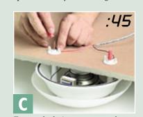
Two standard wire nuts connect the speaker wires to the mounting studs, making the electrical connection.
