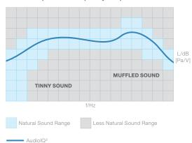
The internal 20-band equalizer in the Plantronics Voyager PRO headset automatically adjusts to background noise to maintain a natural-sounding voice quality. Headsets without Plantronics AudiolQ $^2$  technology tend to sound either too tinny or too muffled.
