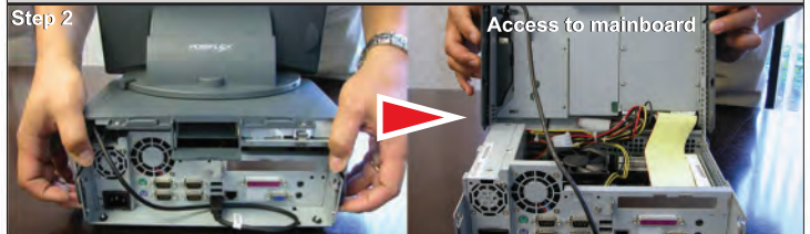
Press buttons on each side of metal chassis and lift system cover
