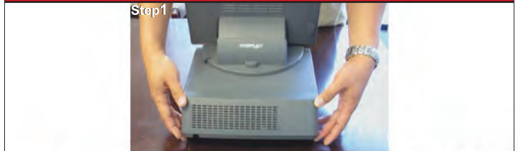
Place finger underneath each corner of rear cable cover and remove
